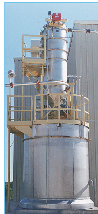
Stainless steel filter receiver
