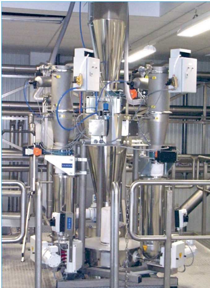
Coperion K-Tron feeders and vacuum conveyors in a continuous food process
