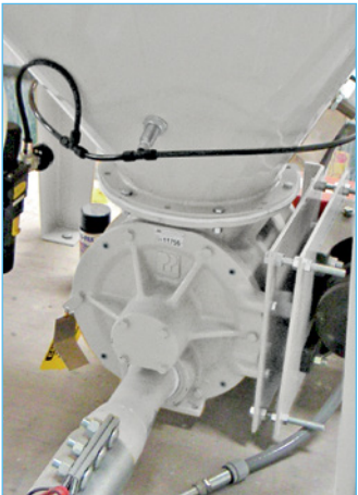
Blow-through rotary valve
